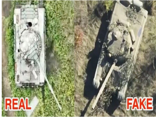
Figure 11: Drone view of Real and Fake Equipment
