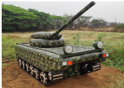
Figure 8: A Decoy Tank Mimicking the Real Asset
