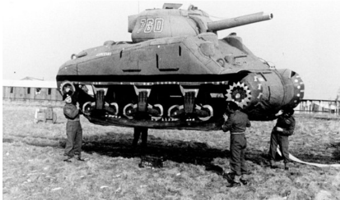
Figure 2: Ghost Army Decoy Tanks Used in Operation Fortitude
